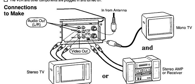
When recording, you may monitor in stereo, by connecting the VCR to either a stereo TV, or a mono sound TV with stereo amp and speakers.
